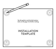
2 Drill into the wall at each marked location. Use a 1/4" drill bit for brick or other masonry wall. Use a 1/16" drill bit for wood wall.
