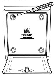
While the mailbox is hanging on the top screws, insert the remaining two screws into the bottom holes and secure with a screwdriver.
