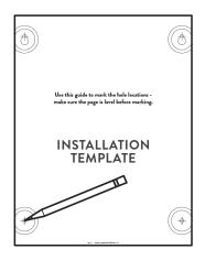
2 Drill into the wall at each marked location. Use a 1/4" drill bit for brick or other masonry wall. Use a 1/16" drill bit for wood wall.
