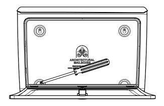
While the mailbox is hanging on the top screws, insert the remaining two screws into the bottom holes and secure with a screwdriver.
