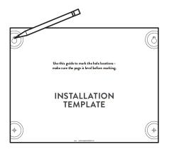
2 Drill into the wall at each marked location. Use a 1/4" drill bit for brick or other masonry wall. Use a 1/16" drill bit for wood wall.
