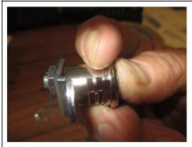
To remove the compartment latch cam, first remove the key from the lock. Due to how easily the core can come loose from the lock body, hold the lock in such a manner that your thumb is pressed against the lock core as you remove the nut.
