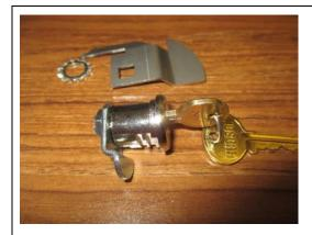
The K30810 Hudson lock kit can be used for compartment doors (as shown with attached cam) or for tenant doors prepared for the USPS lock system. For the latter, the parcel cam shown on top is switched out. Due to the design of this lock, care must be taken to avoid the lock core from separating from the lock body.
