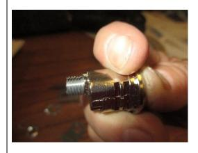
Continue to maintain pressure against the lock core as you insert the lock through the door lock opening. Once you have the lock started through the door opening, you could even grasp the threads of the lock from the inside of the door to keep the lock core in place until you've secured the lock with the provided clip. As you apply the parcel cam, large star washer, and nut, maintain pressure on the lock core from the front once again to keep the lock core in place until the nut is tightened.
