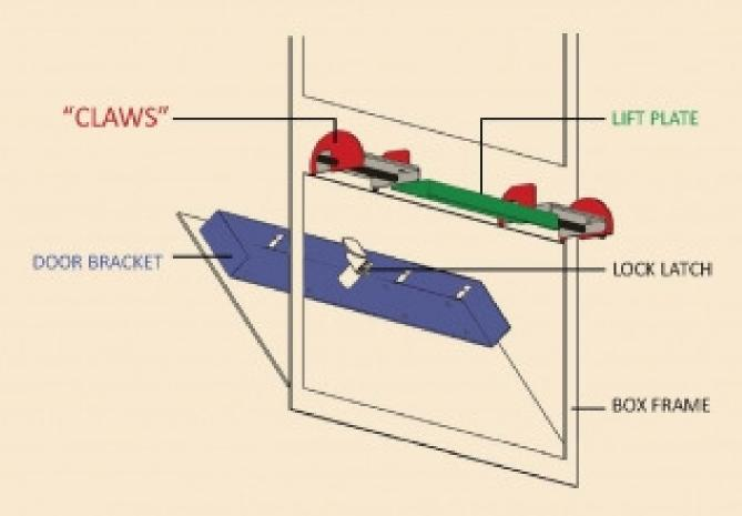
When activated, the Lock Latch pushes up on the Lift Plate which rotates all FOUR stainless steel "CLAWS" into the Door Bracket.
