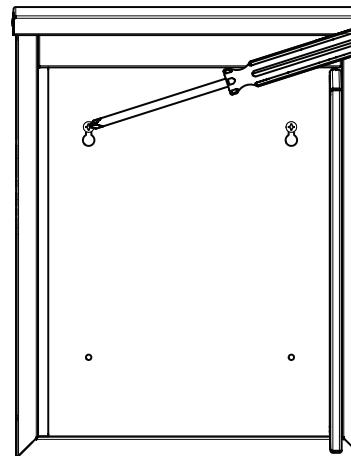
**5** While the mailbox is hanging on the top screws, insert the remaining two screws into the bottom holes and secure with a screwdriver.
