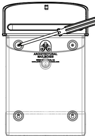
**5** While the mailbox is hanging on the bottom screws, insert the remaining two screws into the top holes and secure with a screwdriver.
