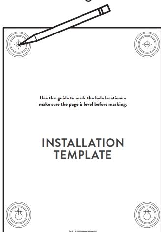
**2** Drill into the wall at each marked location. Use a 1/4" drill bit for brick or other masonry wall. Use a 1/16" drill bit for wood wall.
