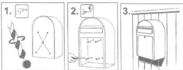
Drill out the 4 preformed holes which are in the back of the mailbox using a  $\frac{1}{4}$ " or 6 mm drillbit.
