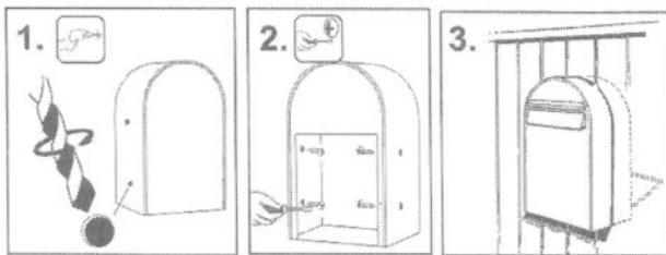
Drill out the 4 preformed holes which are on the side of the mailbox using a  $\frac{1}{4}$ " or 6 mm drillbit.
