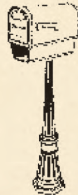
SCC-2008 on SPK-591 Post center mounted
