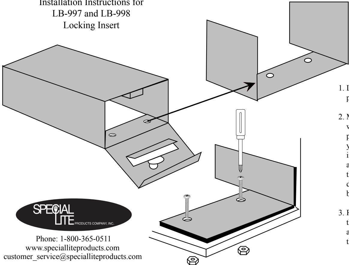
1. Locate holes in bottom plate of locking insert.
