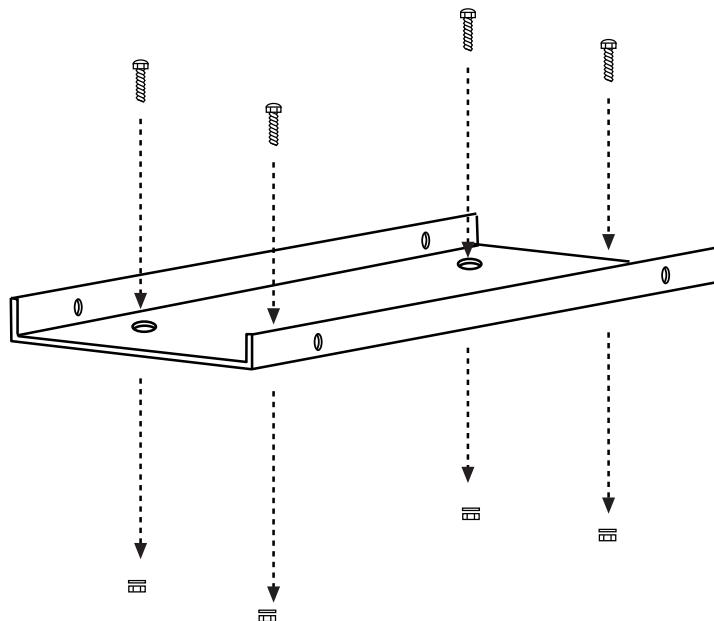
2. Place Mailbox on bracket, aligning side holes. Attach with 4 sheet metal screws
